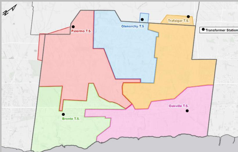
**Figure 2 shows the coverage areas of the high voltage transformer stations that supply electricity to Oakville from 230kV and 115kV transmission circuits. Electricity feeders originating from these stations distribute power at 27,600 volts to customers and substations within the designated colored areas.**
