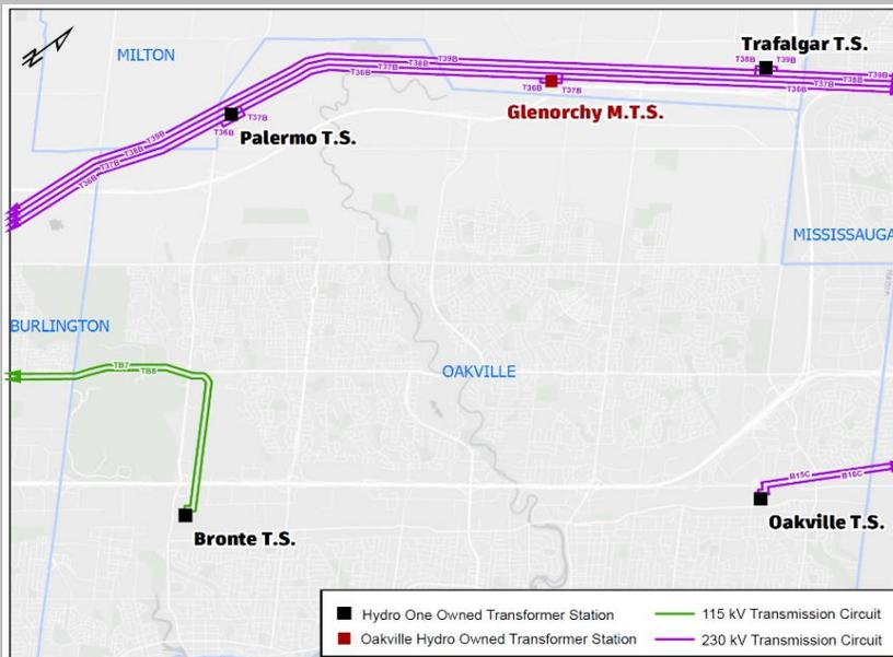
**Figure 1 illustrates Oakville's transmission connections and transformer stations, which convert high-voltage transmission lines to distribution voltages suitable for local delivery. The network comprises three independent high-voltage transmission circuits and five transformer stations, including the Glenorchy Municipal Transformer Station (M.T.S.), which is owned and operated by OH.**
